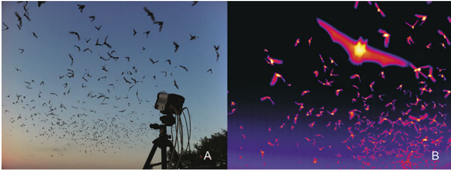
Fig. 8.5 Thermal imaging can be used to produce high-contrast, high-resolution imagery that can be used by a variety of researchers. (a) A visual light image of Tadarida brasiliensis emerging from Frio Cave. Thermal cameras are arranged such that their field of view includes the bats with a backdrop of the sky. (b) The resulting images provide unprecedented detail of bat flight and group behavior (photo credit N.W. Fuller)
